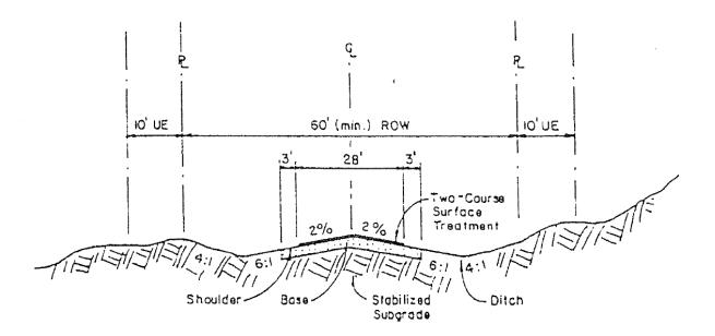
Surface material shall consist of two-course surface treatment comprising of P-3 and P-4 aggregate as TxDOT specifications item 304 at 35#/sy and 15#/sy, respectively and asphalt binder. Surface course shall be laid on prepared and primed flexible base, TxDOT standard specifications for gravel, crushed rock; iron ore) placed on subgrade, both compacted to 95% Modified Proctor. Thickness of base depends on subgrade, material specifications and traffic characteristics.
