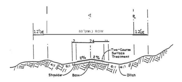
Surface material shall consist of two-course surface treatment comprising of P-3 and P-4 aggregate as TxDOT specifications item 304 at 35#/sy and 15#/sy, respectively and asphalt binder. Surface course shall be laid on prepared and primed flexible base, TxDOT standard specifications for gravel, crushed rock; iron ore) placed on subgrade, both compacted to 95% Modified Proctor. Thickness of base depends on subgrade, material specifications and traffic characteristics.
