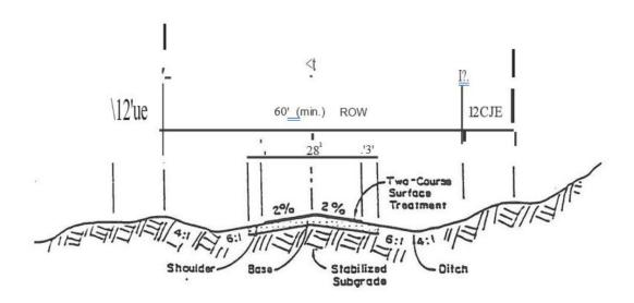
Surface material shall consist of two-course surface treatment comprising of P-3 and P-4 aggregate as TxDOT specifications item 304 at 35#/see and 15#/see, respectively and asphalt binder. Surface course shall be laid on prepared and primed flexible base, TxDOT standard specifications for gravel, crushed rock; iron ore) placed on stabilized subgrade, both compacted to 95% Modified Proctor. Thickness of base depends on subgrade, material specifications and traffic characteristics.
